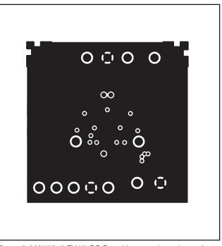
Figure 9. MAX2016 EV Kit PC Board Layout—Inner Layer 2 (GND)
