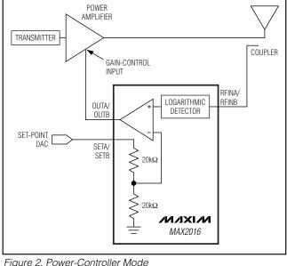
In the power-controller mode (Figure 2), the DC voltage at OUTA or OUTB controls the gain of the PA leading to a constant output power level. (Note: Only one controller channel is shown within the figure. Since the MAX2016 is a dual controller/detector, the second channel can be easily implemented by using the adjacent set of input and output connections).
