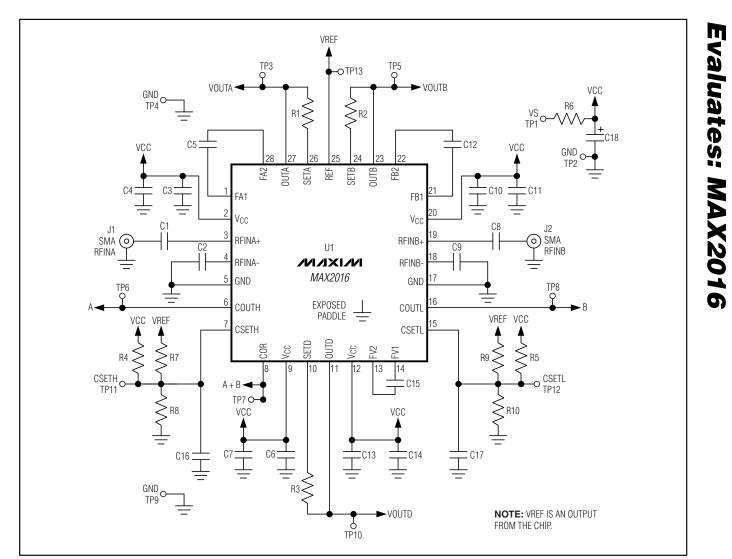
Figure 4. MAX2016 EV Kit Schematic
