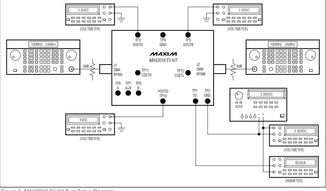
Figure 1. MAX2016 EV Kit Test Setup Diagram
