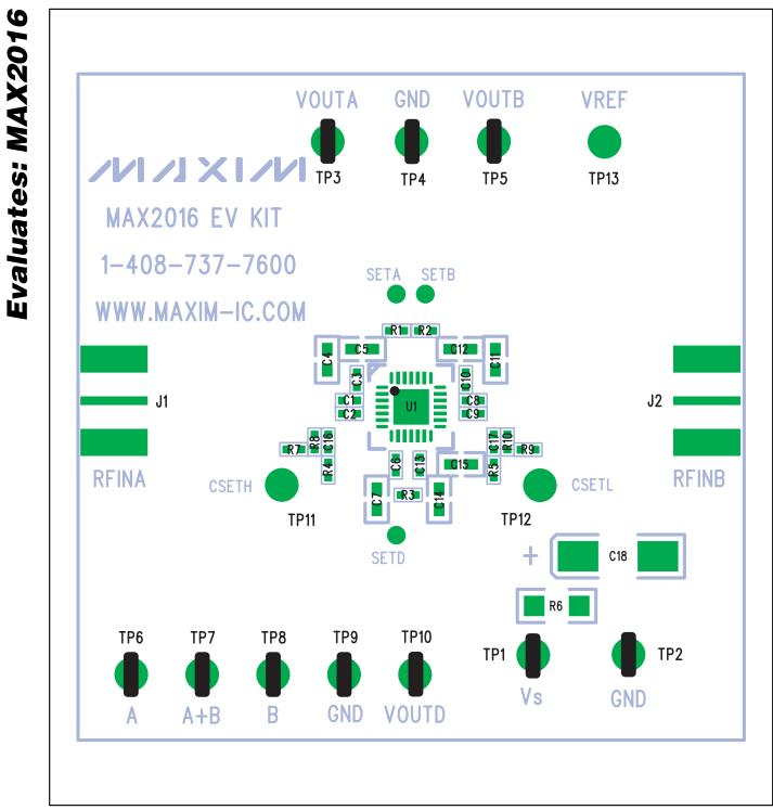
Figure 5. MAX2016 EV Kit Component Place Guide—Component Side
