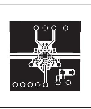
Figure 8. MAX2016 EV Kit PC Board Layout—Top Layer Metal
