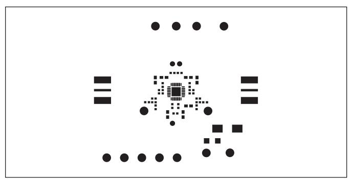
Figure 7. MAX2016 EV Kit PC Board Layout—Top Solder Mask
