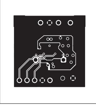
Figure 10. MAX2016 EV Kit PC Board Layout—Inner Layer 3 (Routes)
