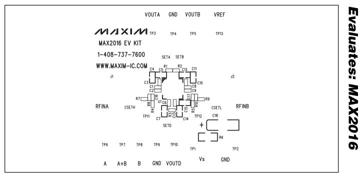
Figure 6. MAX2016 EV Kit PC Board Layout—Top Silkscreen
